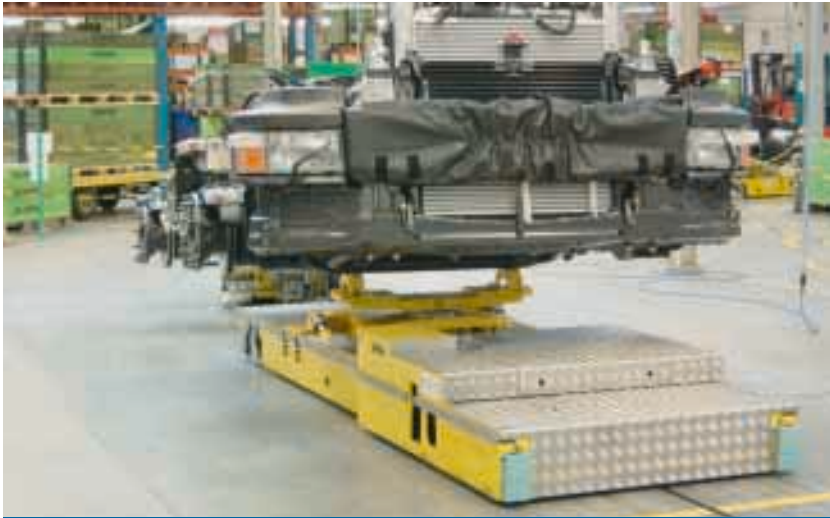
Transporting trucks on an inductive floor conveying system.
